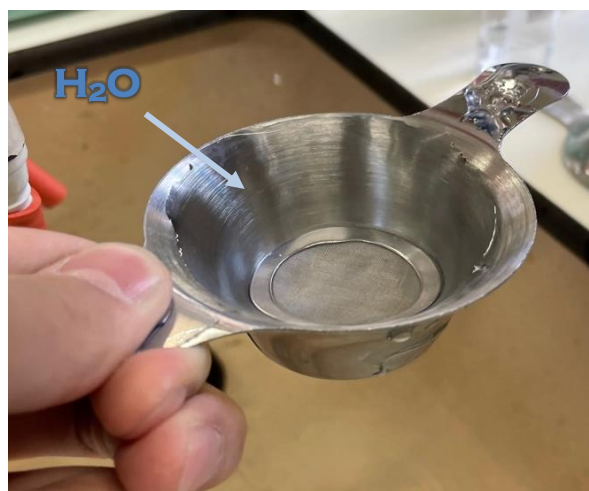
Figure 1b: Checking waterproofing of an alginate-coated sieve
