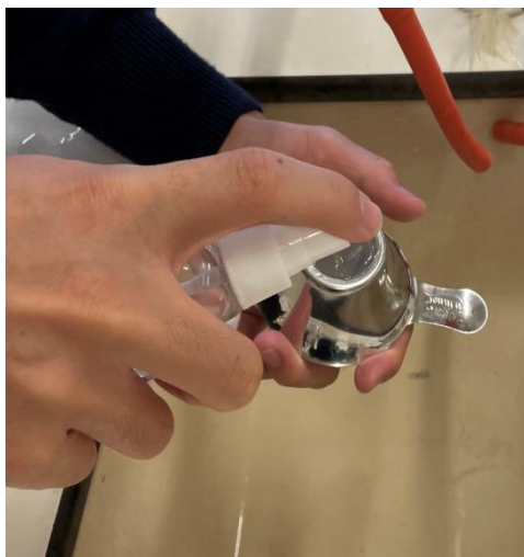
Figure 1a: Spraying \text{Ca}(\text{NO}_3)_2(\text{aq}) to a sieve
